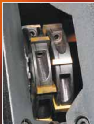
2 milling disks and 6 pcs. high speed indexable inserts
