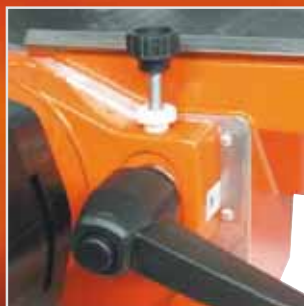
Fine Adjustment of Milling Depth/Bevel Width
