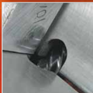
Exact Deburring by means of self-generating milling cutter
