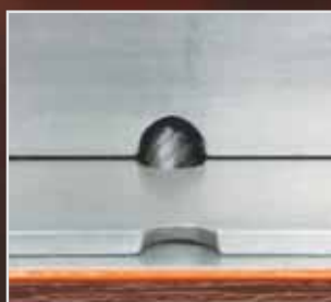
Position II: Material thicknesses as from 1.0 mm
